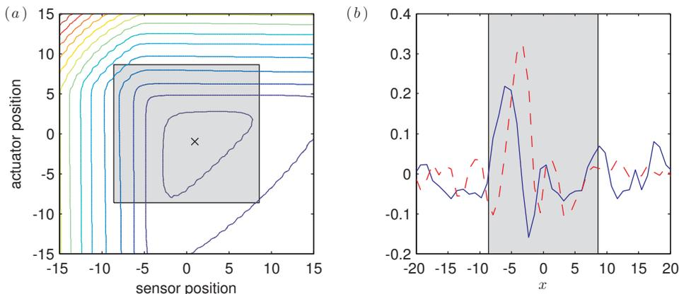
FIGURE 2. (a) Contours of  $\log_{10} \gamma_2$  and the optimal placement ( $\times$ ), with disturbances introduced everywhere. The innermost contour is  $\log_{10} \gamma_2 = 2$ , and each subsequent contour increments by 0.5. (b) A sample snapshot of the controlled perturbation  $q$ , shown as real (solid/blue) and imaginary (dashed/red) parts. The actuator is at  $x_a = -1.00$  and the sensor is at  $x_s = 1.00$ . In both plots, the region of amplification is shaded grey.
