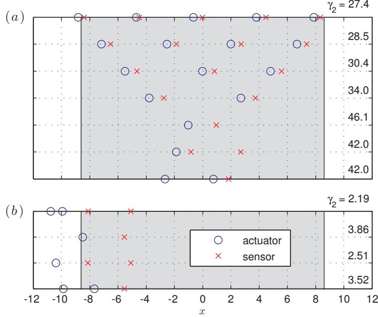
FIGURE 4. Optimal placement for different numbers of actuators and sensors. The  $H_2$  norm  $\gamma_2$  is tabulated for each configuration, and the region of amplification is shaded grey. (a): Disturbances present everywhere. (b): Disturbances introduced at  $x_d = -11.0$ .
