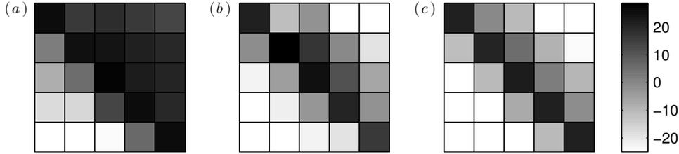
FIGURE 5. The LQG gain in the optimally-placed five-input, five-output system, shown in decibels. The block in row  $j$  and column  $k$  shows the gain from a signal  $\exp(i\omega t)$  in sensor  $k$  to actuator  $j$ , assuming that the sensors and actuators are ordered from upstream to downstream. (a): At  $\omega = 10^{-1}$ ; (b): at  $\omega = 10^1$ ; (c): at  $\omega = 10^3$ .
