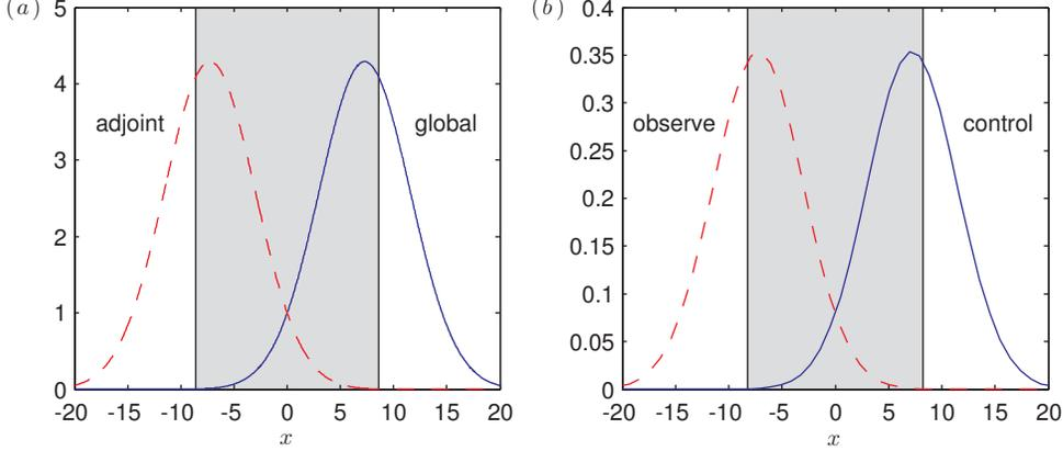
FIGURE 6. (a): Leading global and adjoint eigenmode magnitudes, for  $\mu_0 = 1.03\mu_c$ . (b): Leading modes of the observability and controllability Gramians (assuming full sensing and actuation), for  $\mu_0 = 0.96\mu_c$ . The region of amplification is shaded grey.
