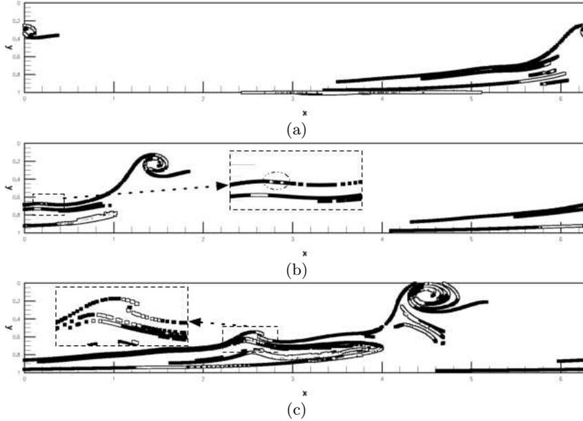
FIGURE 6. Magnitude of  $\langle \mathbf{n}, \mathbf{S}\mathbf{n} \rangle$  along spanwise-constant cross sections of LCS surfaces at times (a)  $t^+ = 45$ , (b)  $t^+ = 63$ , and (c)  $t^+ = 99$ . Negative strain rate (compression normal to the surface) is black; positive strain rate (expansion) is white with black outline.
