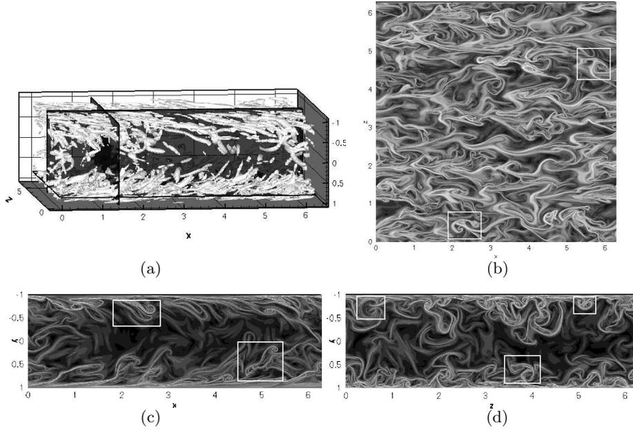
FIGURE 7. Two dimensional DLE plots of the fully turbulent channel. (a) 1% max  $Q$  superimposed with location of the three planes, (b) constant wall-normal cut, (c) constant-spanwise cut ( $y^+ = 33$ ), and (d) constant-streamwise cut
