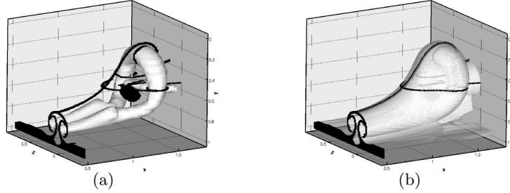
FIGURE 4. (a) Isosurfaces of 10% max  $\lambda_{ci}^2$  (white) superimposed on three planes of DLE  $\geq 60\%$  max (black); (b) Translucent isosurfaces of 60% max DLE (white) superimposed on three planes of DLE  $\geq 60\%$  max (black)
