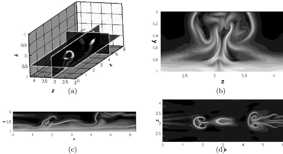
FIGURE 5. Two dimensional DLE plots of the isolated hairpin evolved to  $t^+ = 171$ . (a) 10% max  $\lambda_{ci}^2$  superimposed with location of the three planes, (b) constant-streamwise cut, (c) constant-spanwise cut, and (d) constant wall-normal cut ( $y^+ = 95$ )
