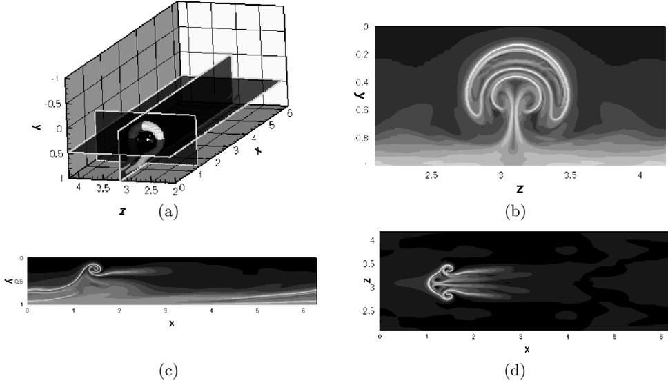
FIGURE 3. Two dimensional DLE plots of the isolated hairpin evolved to  $t^+ = 63$ . (a) 10% max  $\lambda_{ci}^2$  superimposed with location of the three planes, (b) constant-streamwise cut, (c) constant-spanwise cut, and (d) constant wall-normal cut ( $y^+ = 98$ )
